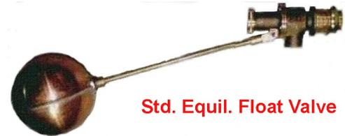
The most common type in use within the UK domestic market is the 15mm BS 1212 type as applied to most domestic W/Cs and loft tanks. BS 1212 Valves are more restrictive on flow and incur a much higher headloss than say those of the Equilibrium type. For intermittent use this is satisfactory. However with ever reducing mains pressures, tanks that are in constant demand require the lower head loss and higher capacity benefits of the Equilibrium type.
