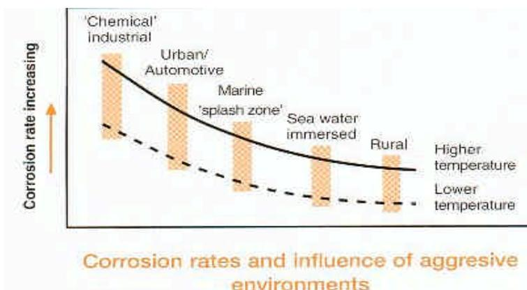
For many aqueous reactions a 30 deg. C temperature change results in a 10 fold change in corrosion rate, while a 20 deg. C change will approximately double the corrosion rate.
