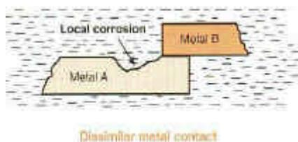
This is particularly damaging if the more 'active' (anodic) metal has a smaller area.
