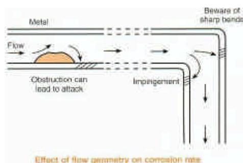
The flow of fluids relative to a metal can increase the corrosion rate. Erosion corrosion may become significant at high rates of flow when the flow changes from laminar to turbulent.
